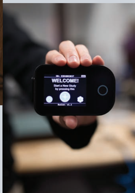
↓ Able to record a patient’s heart rhythm for up to 30 days, the Clarus 40M can also detect common arrhythmias and wirelessly transmit that information to medical staff.
