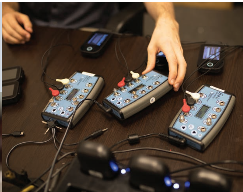
↑ Before releasing the latest version of a product, engineers at TZ Medical test firmware changes in the updated device using simulated ECG signals. Here, an engineer tests the Clarus 40M cardiac monitor.
