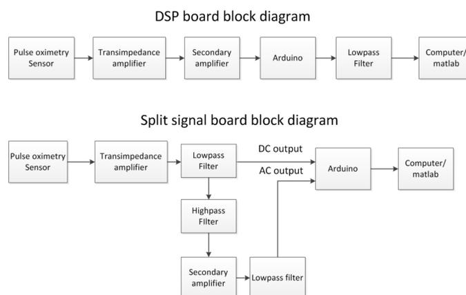
Figure 3. Block diagrams for the DSP and the split signal boards.
