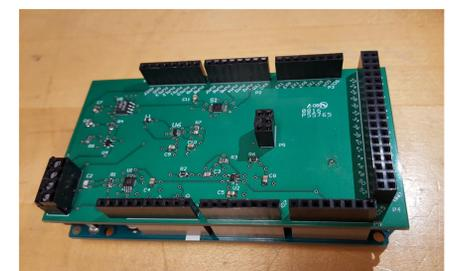
Figure 8. Split signal hardware filter board
