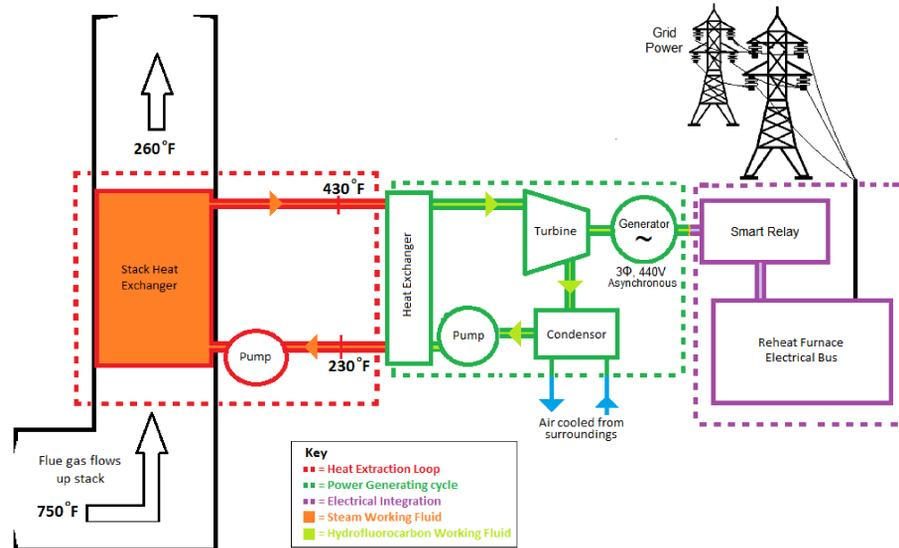
Figure 2. The Waste Heat Recovery System
