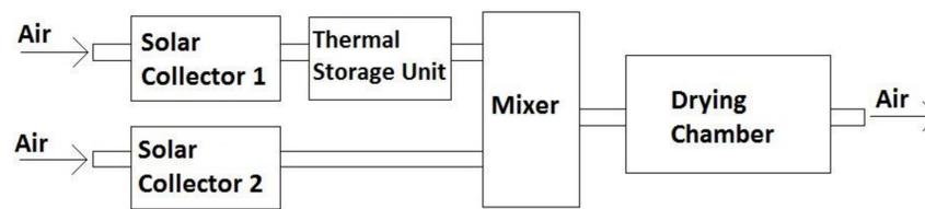
Figure 2. Block diagram of the system.
