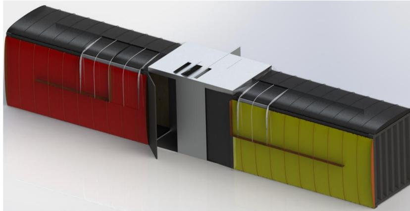
Figure 3. The final design of the solar dryer system, which includes the thermal storage unit (left, in red), the mixer unit (center, in grey), and the drying chamber (right, in yellow).
