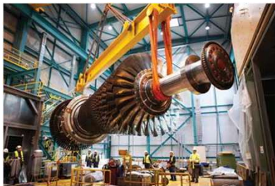
Figure 1. Power Turbine During Maintenance
