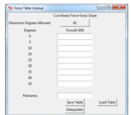
Figure 9. GUI used to adjust sway tolerances
