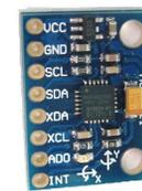
Figure 7. MPU6050 utilized to detect test subject sway
