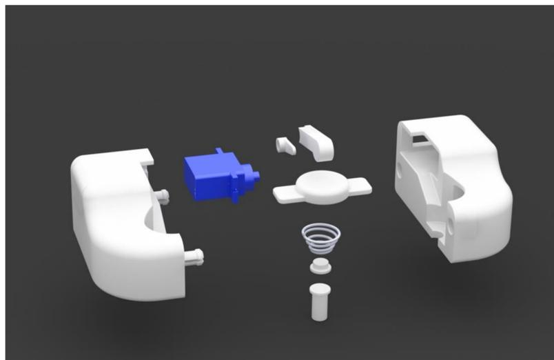
Figure 5. Exploded view of the button with the servo motor, spring mechanism
