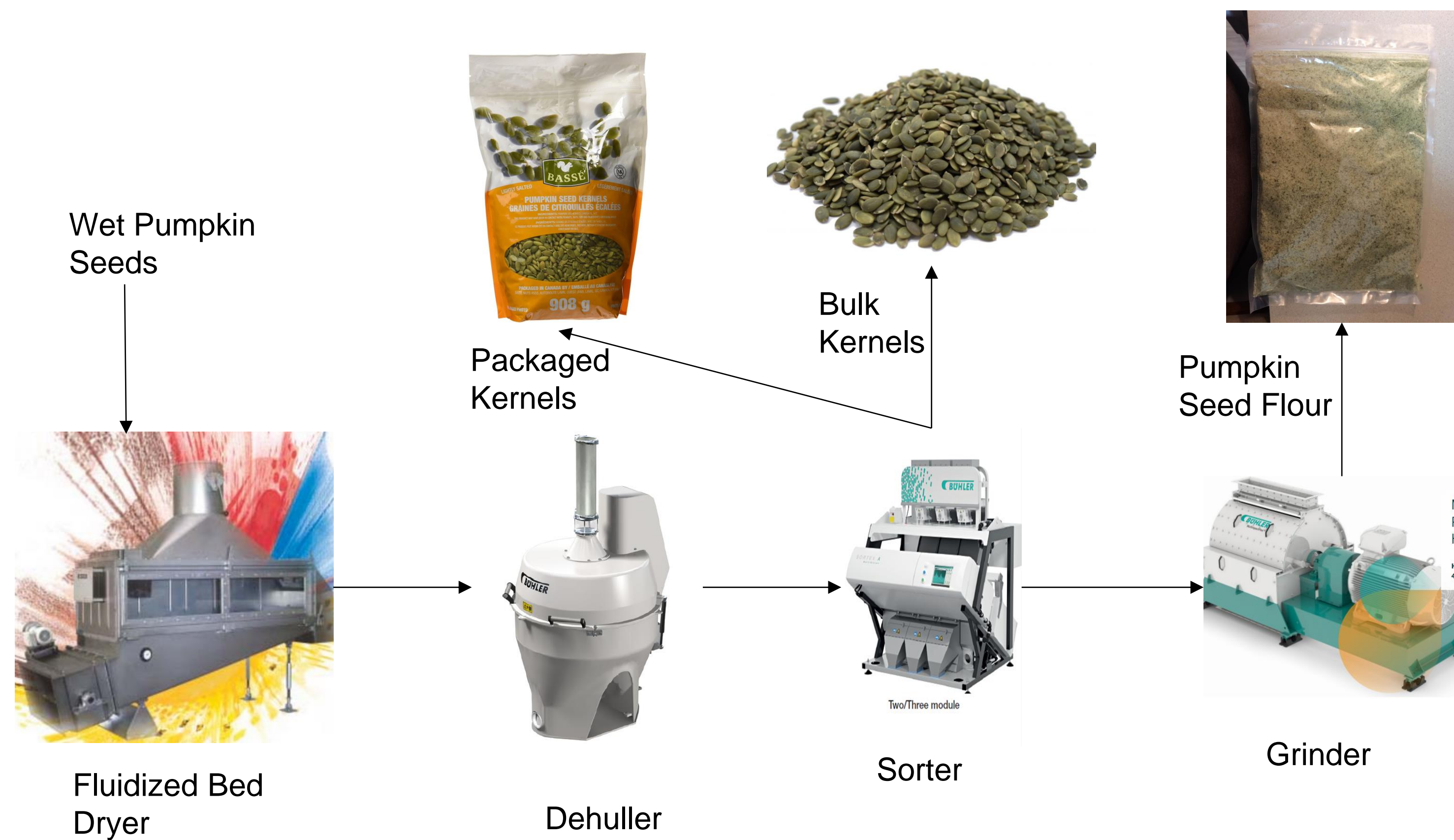
Figure 4 : Pumpkin Seed Processing Line
