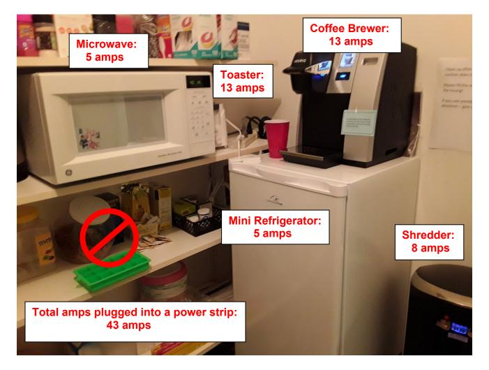
Do NOT overload circuits. (The above picture is of an overloaded electrical circuit.) Most circuits run about 15-20 amps. The general rule is to use 80% (16 amps) of that circuit.
